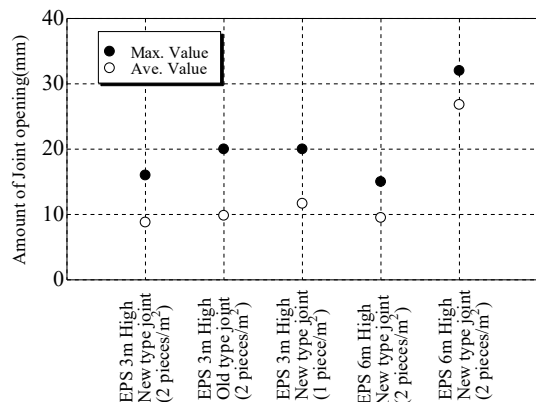
Fig. 4. Amount of opening between blocks after shaking test (performance comparison of metal)
